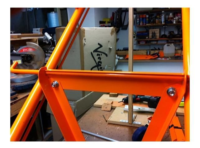
Now attach the Cargo Bar to the drilled lugs on the lower section of the trolley's shafts, using the four bolt and but assemblies provided.
