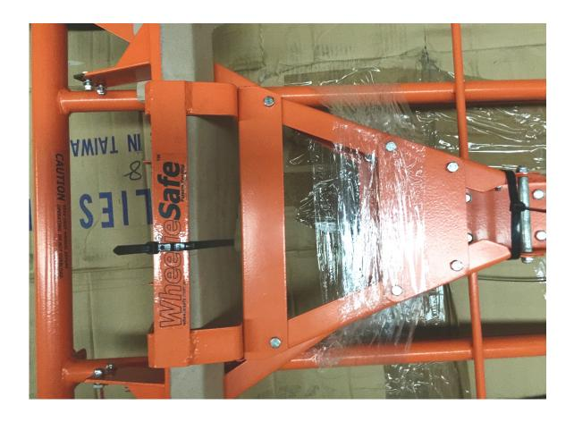
Cut the two electrical ties and lift out the Handling Bracket and the Cargo Bar.
