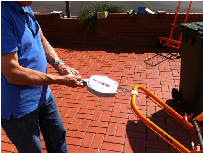
Using the Wedderburn scale to test pull force
