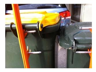
When bins of equal or unequal size place the smaller bin slightly behind the larger bin. The larger bins should be loaded on the top hook closest to the shaft and the smaller bin on the lower hook closest to the shaft. When the bins are loaded the Bin Retaining Pillars will locate against the face of the bin handle bar bracket as shown. The pillars are of different lengths to accommodate different sized bins.
