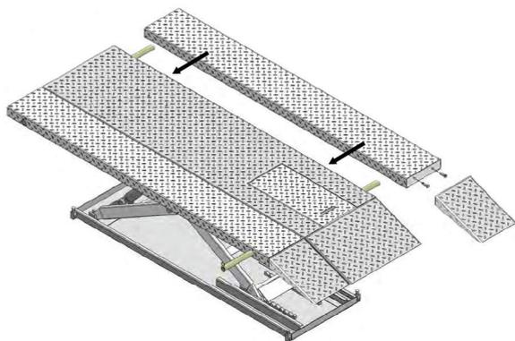
An example of Hospital Bed Maintenance Lift with the Width Extension Kit, adding 300 mm to each side.
